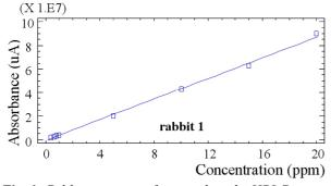
Fig. 1. Calibration curve for parathion by HPLC
